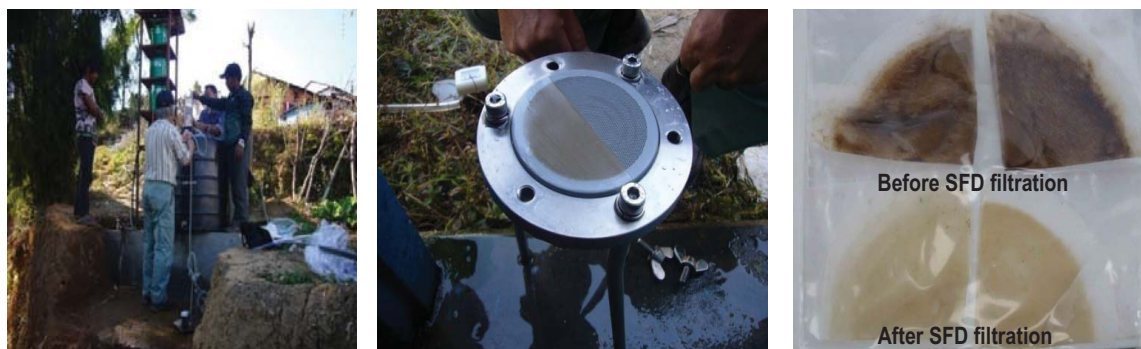
Fig. 4: Bacteriological checking of water (left), membrane filtration device (with PTFE membrane filter) (center) and membrane filters (before and after SFD filtration) (right)
