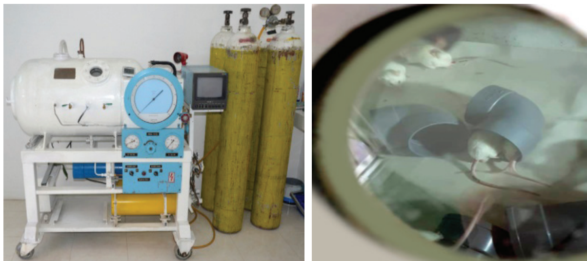
Fig. 1: Chamber designed and used of the exposure of HBO (left) and mice being exposed to HBO in the animal chamber (right)
